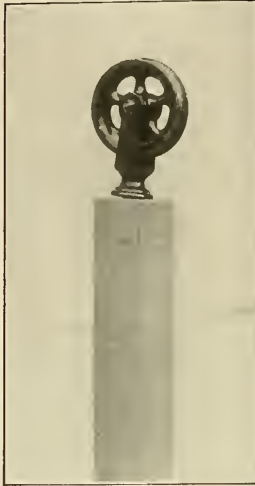
Fig. 572.—Pulley arranged on broom-handle to be fastened at foot of bed for carrying extension cord.
